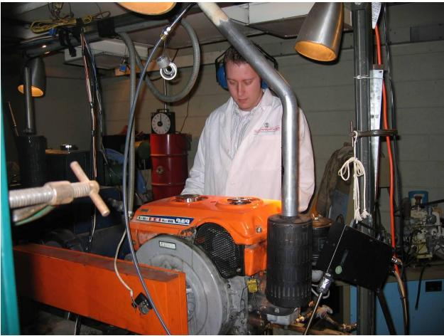
Engines are equipped with dual-fuel system, fuel feed is switched from diesel to test fuel during starting sequence
