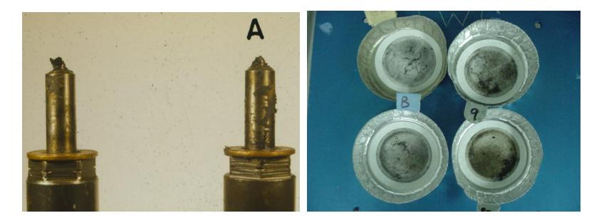
Alternative fuel coking is normalized to #2 diesel fuel Diesel Fuel Coking Index = 1 Lower Index = Better Performance
