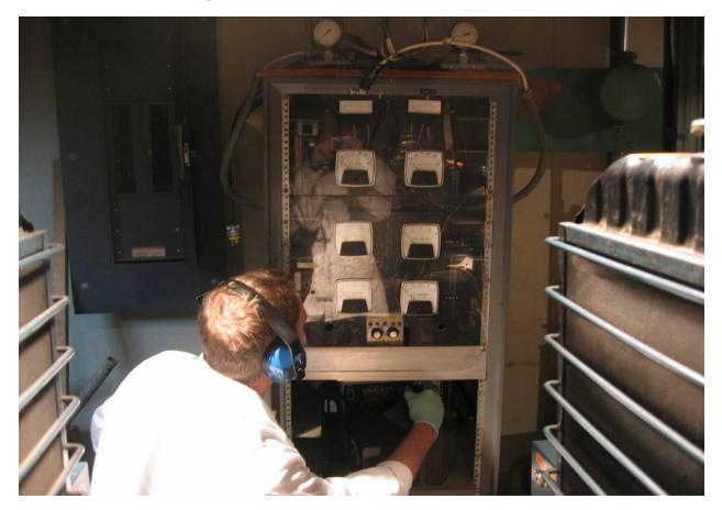
Engines are loaded by dumping current from generator into resistor bank. Increased resistance = increased power output Peterson Test leads to accelerated engine wear
