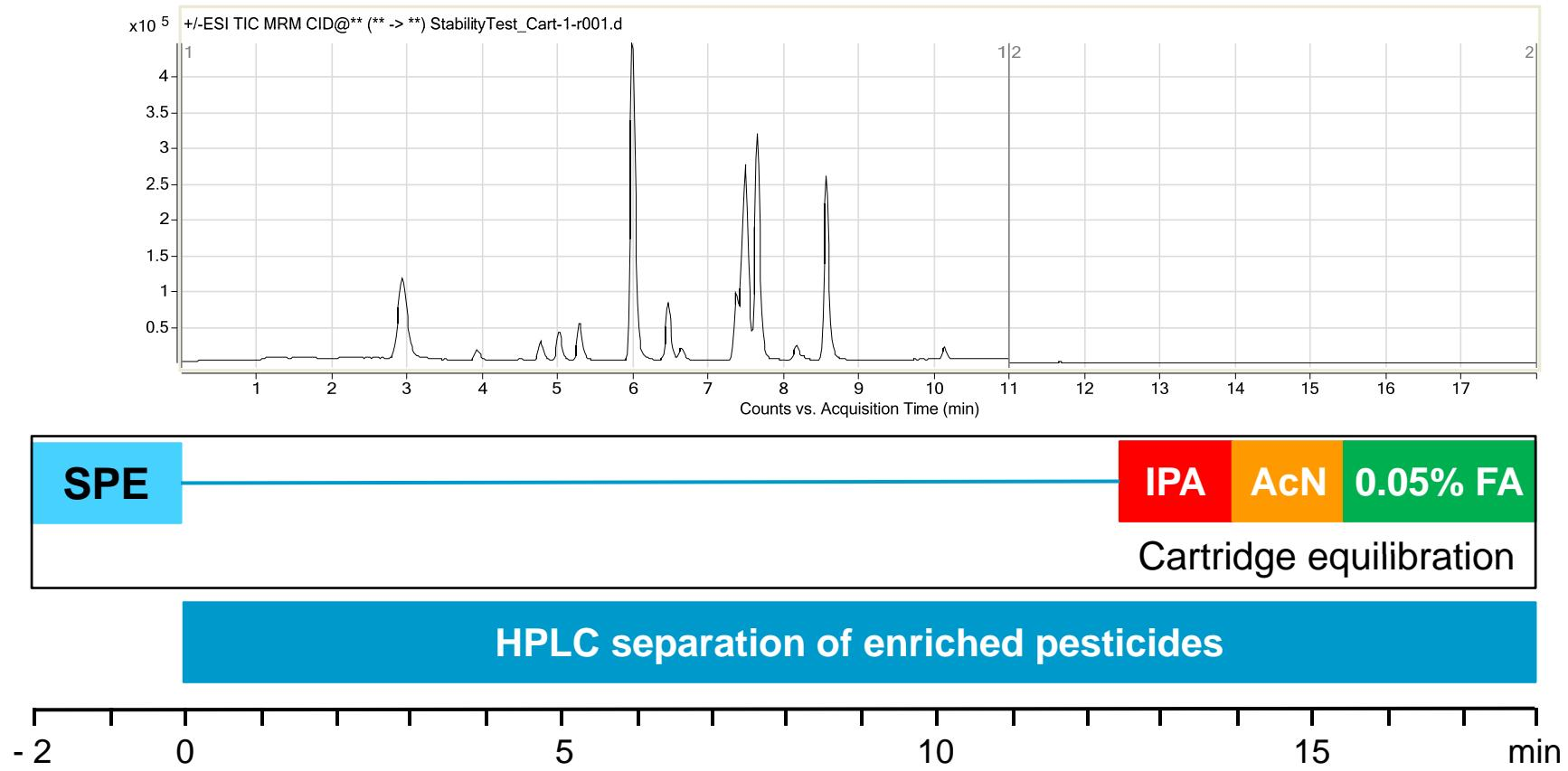
Equilibration of SPE cartridges, SPE and separation of pesticides is overlapped and results in a total runtime for the method of 20 minutes.
