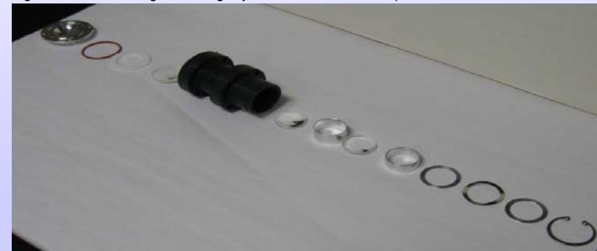
Figure 3. Individual components as assembled in the FM-3001 FPD MINICAMS coupling assembly
