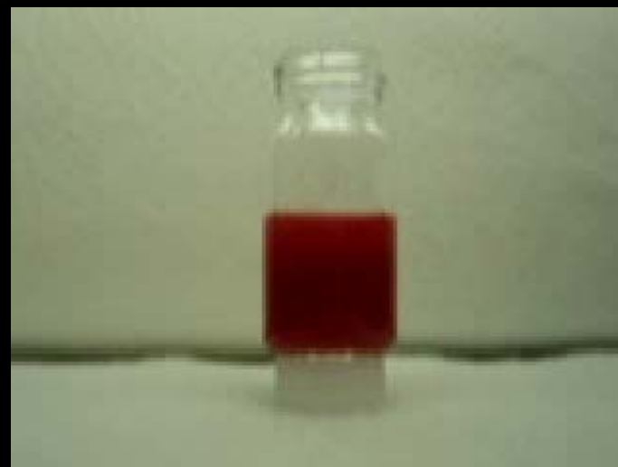
1ppm SeCN Solution 2 min after HNO 3 addition
