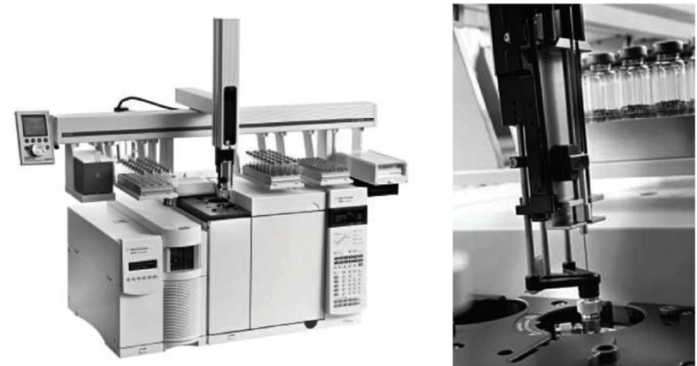
Figure 3.1 Automated GC SPME analysis with expansion of the SPME injection. Reproduced with permission from GERSTEL GmbH & Co. KG
