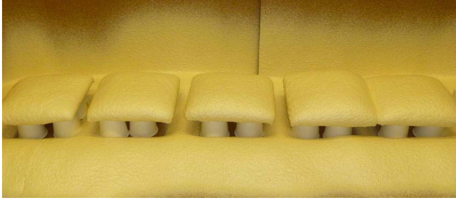
Five replicate closed-cell SPF samples are shown in the spray booth.
