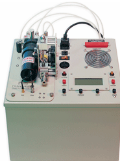
Flame photometric detector (FPD) MINICAMS®
