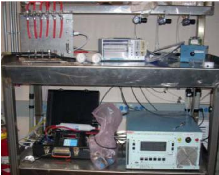
Automatic Continuous Air Monitoring System (ACAMS) ↑
