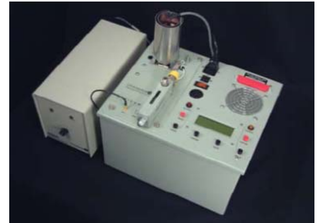
Halogen specific detector (XSD) MINICAMS®
