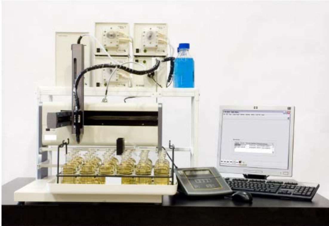
Figure 1. Fully automated system for Seed, inhibitor and dilution water addition. These options are also available without the autosampler.
