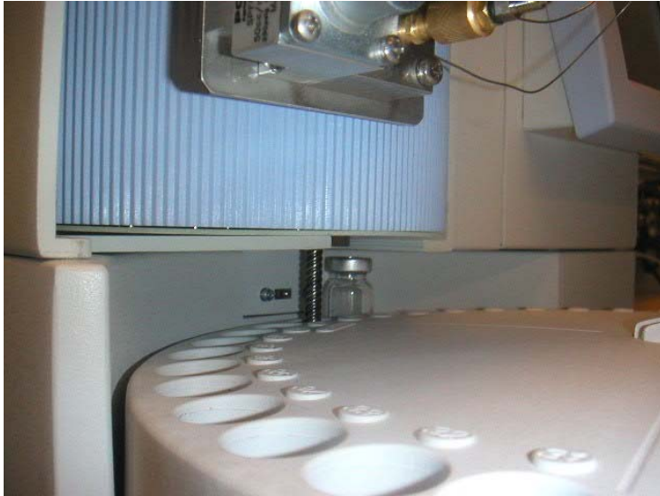
Figure 2. Headspace unit used to precisely introduce mercury vapor.
