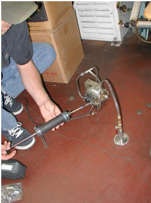
Farallon technician measures VOCs in soil vapor using a detector tube.
